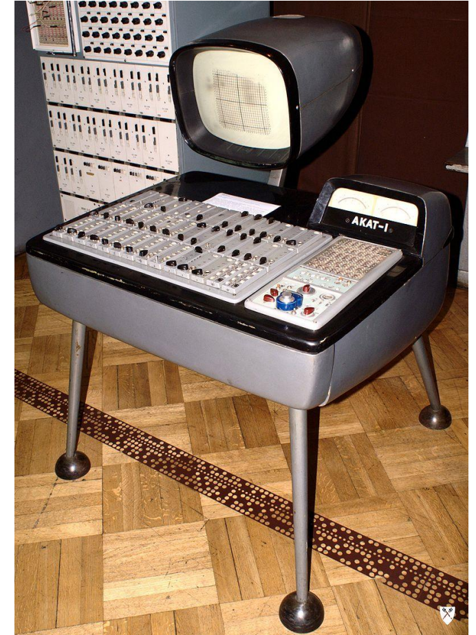
Polish analog computer AKAT-1 (1959) Source: Topory
